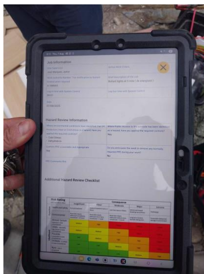
A field tablet on site, mid-task, with the workflow open: hazard review, PPE confirmation and risk matrix at the point of decision.
